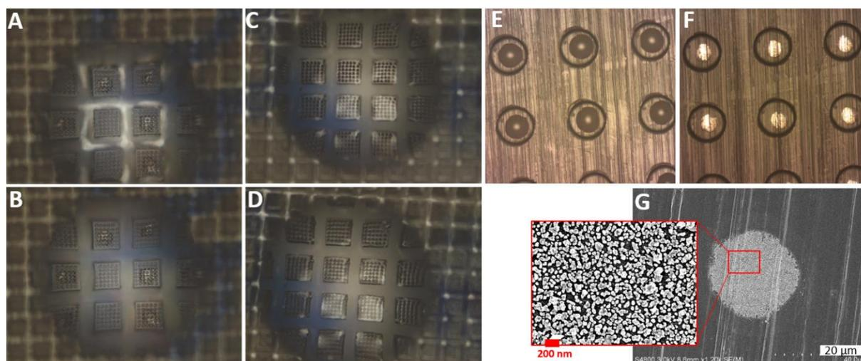
**Figure 1:** Comparison of optical microscopic images of a water droplet on different surface structures after (A and C) 30 s and (B and D) 5 min. Optical microscopic images of (E) deposited silver precursor and (F) sintered silver nanoparticle patterns. (G) SEM images of sintered silver nanoparticle pattern.
