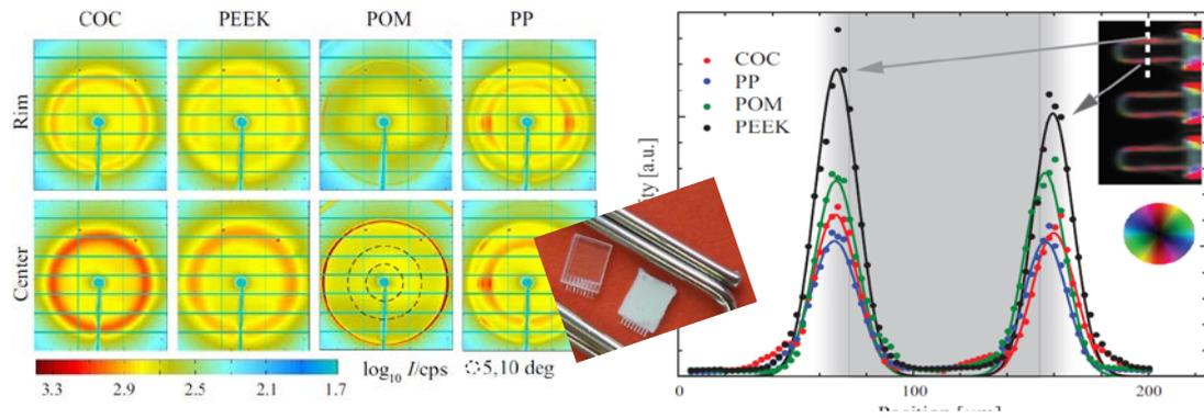
Fig. 1: WAXS patterns of micro-injection moulded cantilevers (left) and SAXS (right), taken at the “Swiss Light Source” (from Ref 4).
