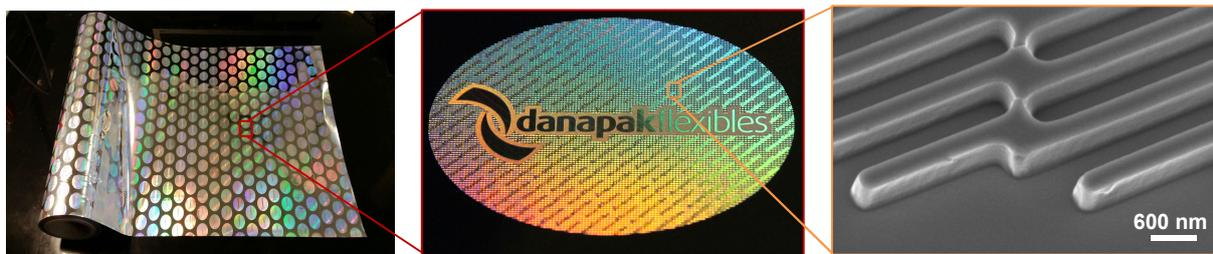
**Figure 2:** Photo of a single layer foil presenting a holographic logo for Danapak flexibles A/S (left), a magnified photo (center), and a respective SEM showing an about 500 nm wide and 650 nm high line grating in PP (right).
