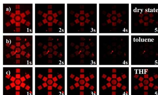
Fig. 4: Fluorescence decay of spiropyran-functionalized structures in different solvents after initial activation with UV-light
