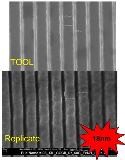
Fig. 2: 18nm wide, >20nm deep channels formed by micro-IM in PP. Tool: HSQ lines on Si, made by EUV-IL at PSI.
