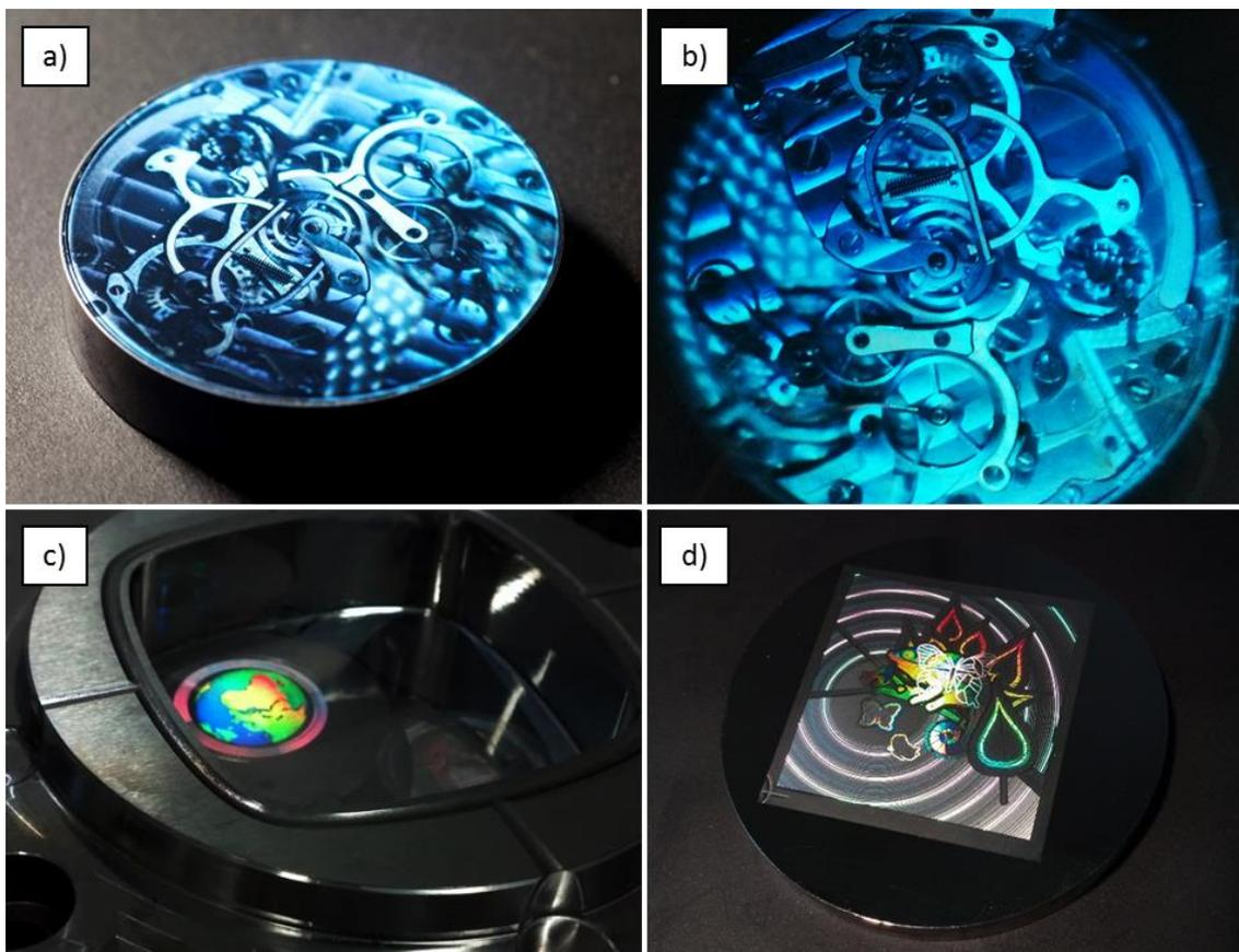
**Figure 1:** a) multilevel hologram in steel, b) hologram molded into black plastic, c) security hologram on the bottom of a steel cavity for injection molding, d) “alphagram” in steel (cooperation with Surys).
