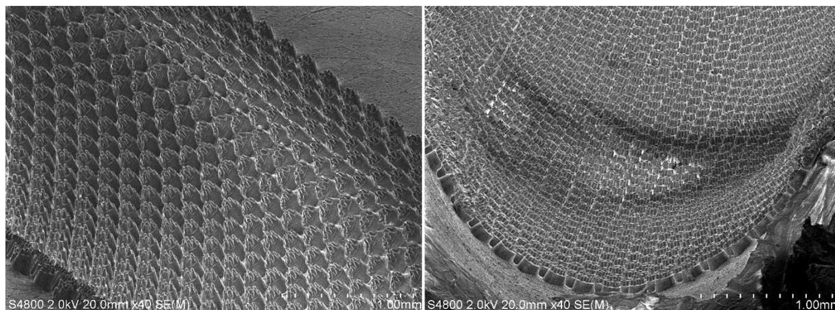
**Figure 1:** Groove-shaped hierarchically micro–micro structured polypropylene surface depicted from two different angles of view.
