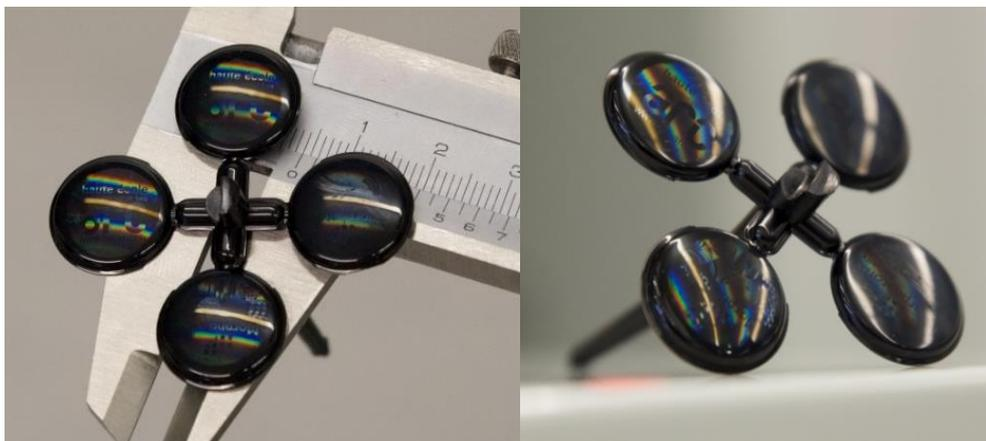
**Figure 1:** Injection molded curved "pills" with diffractive security elements replicated from nano-engraved steel tools
