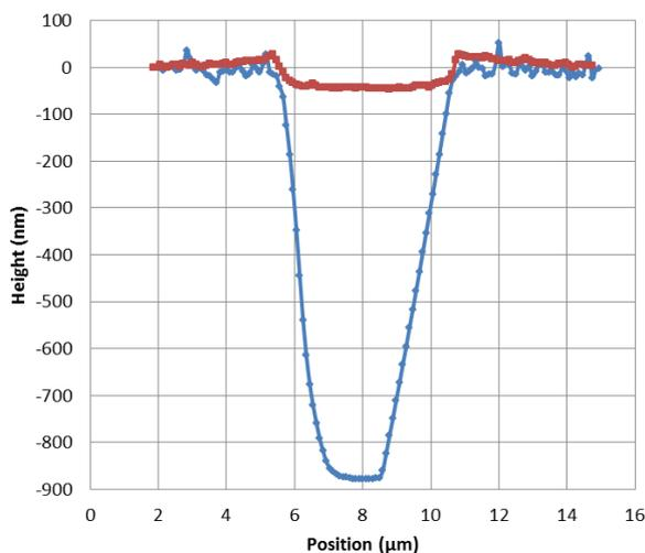
Figure 3: AFM measurement of a mould mark (blue) and how the mark was replicated by the polymer (red).
