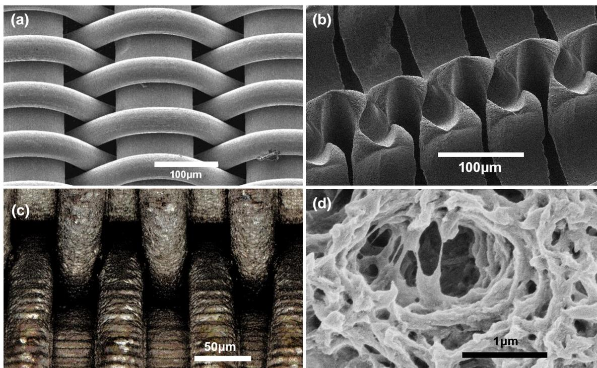
**Figure 1:** SEM pictures of a) wirecloth used as embossing stamp, b) surface structure after hot embossing wirecloth in PP, c) CLSM image of laser treated wirecloth and d) SEM image of PP after swelling in Heptane/Cyclohexane solution
