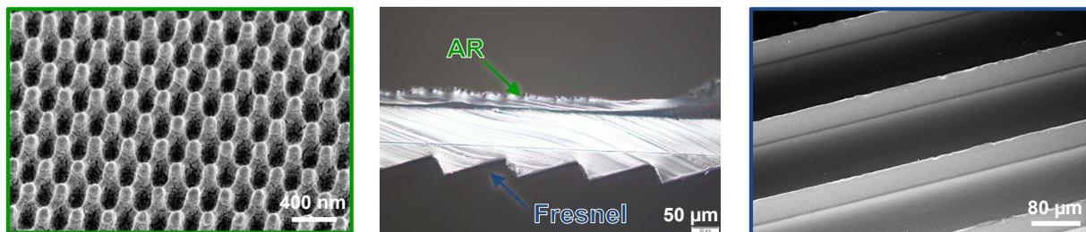
**Figure 1:** SEM of an antireflective structure in polypropylene (PP) (left, masters made by Temicon GmbH), light microscope image of a multilayer foil consisting of PP/PET/PP (center), and SEM of Fresnel lens microstructures (right).
