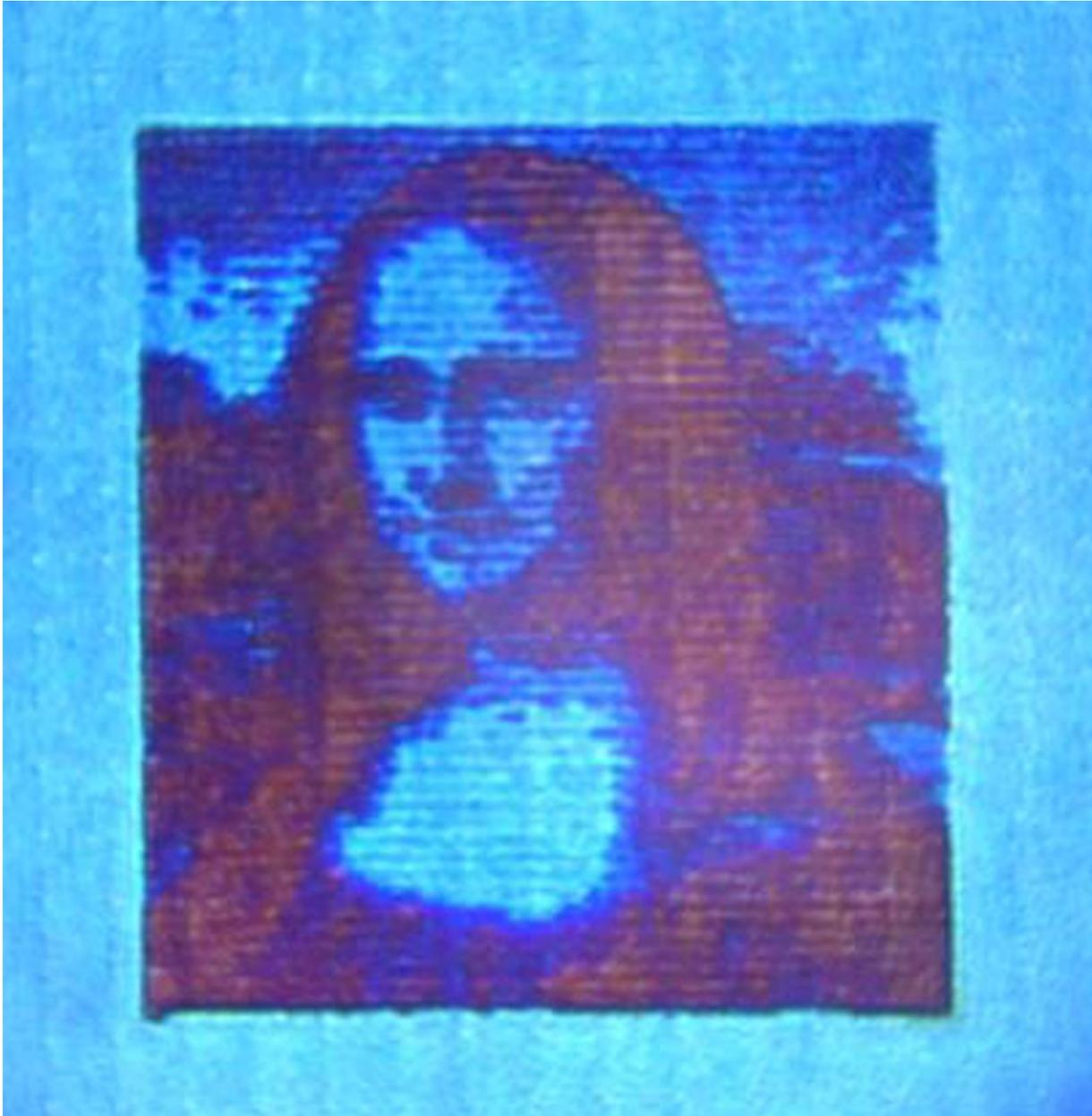
**Figure 1:** The world smallest laser printed Mona Lisa – printed by plasmonic laser printing. The picture is  $50 \times 50 \mu\text{m}^2$  and fits into a single pixel on your iPhone's retina screen.
