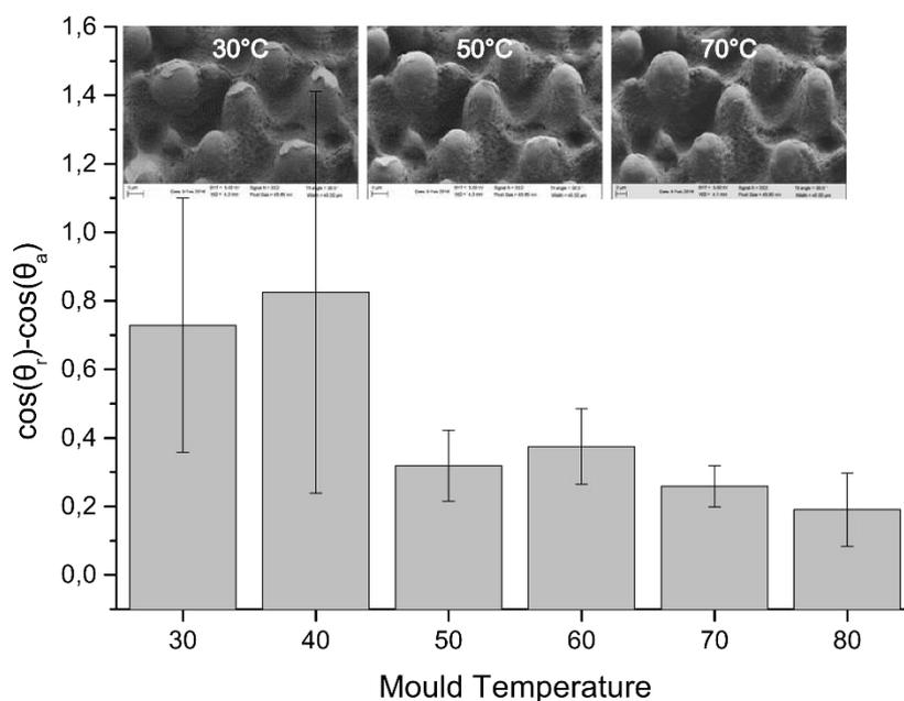
**Figure 1:** Contact angle hysteresis of surfaces for different moulding temperatures. At 50°C degrees, moulding temperature there is a drastic drop in hysteresis indicating the Cassie Baxter state
