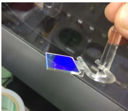
Figure 1: A nanoinjection molded lens with anti-reflection structures on both sides. When looked at glancing angles, it strongly reflects the blue and smaller wavelengths. The light transmission through the lens is >95% leading to high clarity, reduced UV transmission and lower stray reflection.
