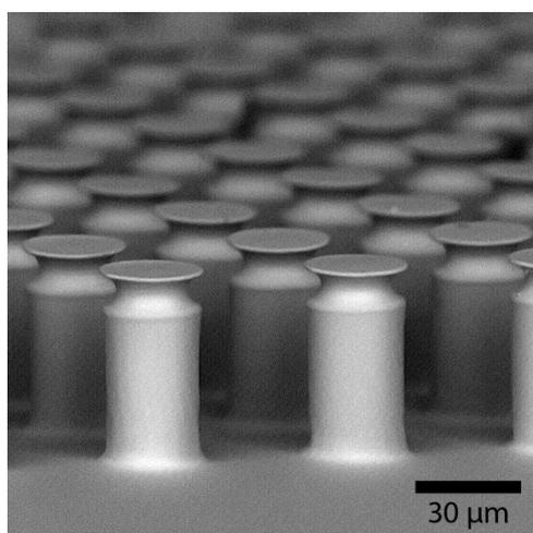
**Figure 1:** Scanning electron micrograph of fibrillar dry adhesive fabricated via two-photon lithography and subsequent replication into elastomeric material.
