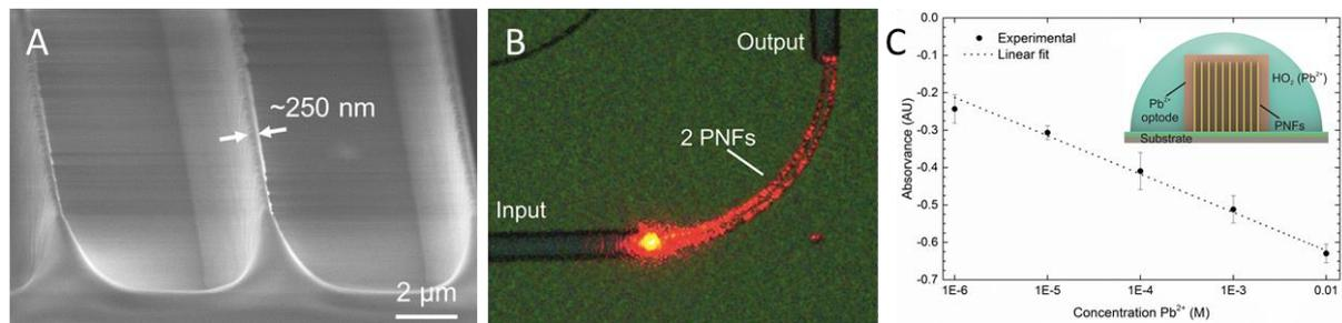
**Figure 2:** (A) SEM image of a photonic nanofence with HAR ~40. (B) Picture of the light coupling from an input waveguide into a 2 PNFs array with bent shape. (C) Calibration curve of a PNF-based lead (Pb) sensor. The inset shows a cross-section schema of the sensor.
