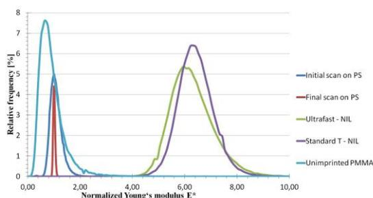
**Figure 2:** Relative modulus of PMMA with/without imprint. The two broad peaks on the right side are representing the normalized Young's modulus for ultrafast NIL and for standard T-NIL for PMMA while the group of peaks on the left side represents the pristine PMMA without imprinting as well as the PS reference measurements before and at the end of the measurements.
