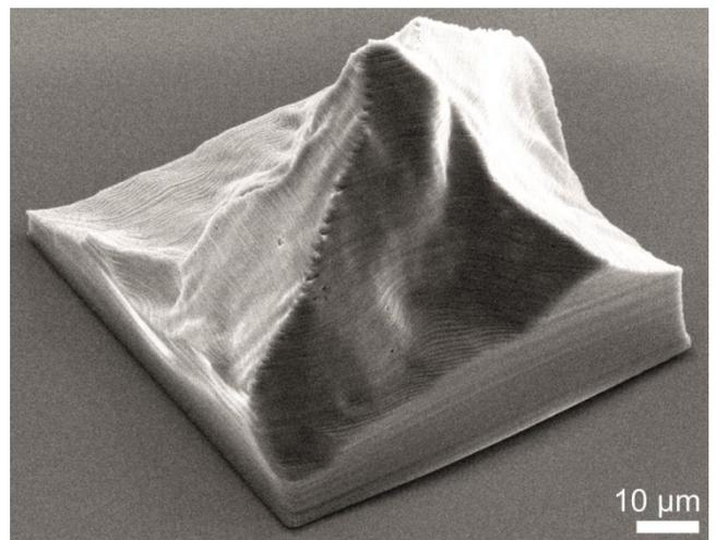
Fig. 5: 3D-printed “Micro-Matterhorn”, taken from ref. 6.
