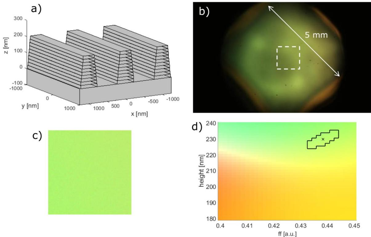
**Figure 1:** **a)** Illustration of the simulation setup for a line grating. **b)** Color image of sample with line gratings, white square represent analyzed region. **c)** Cropped region from b), with colors scaled to correct non-uniform light intensities. **d)** Output from the fitting process. Each color corresponds to a simulation with different heights and filling factors. The black cross is the optimum fit, while the surrounding black lines indicate the 95% confidence limits.
