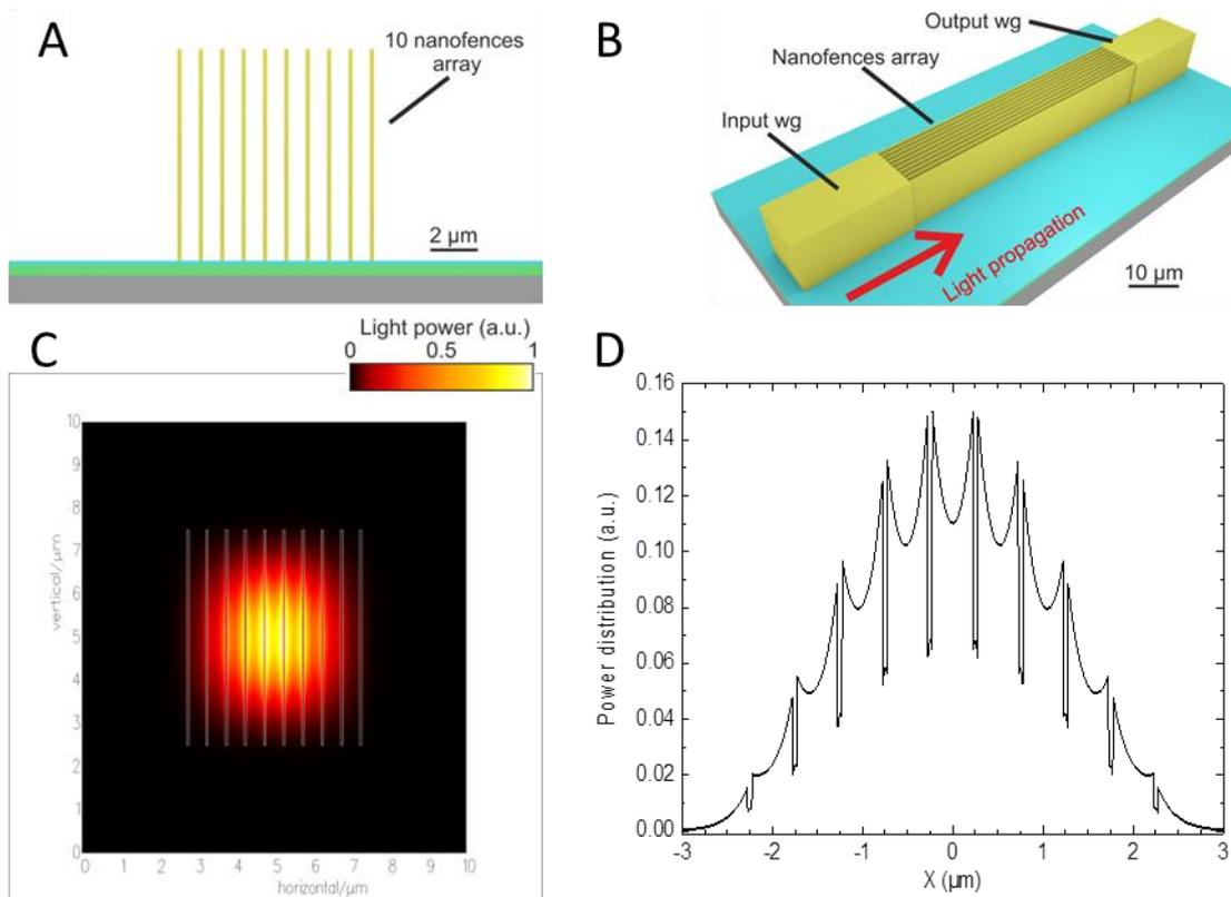
**Figure 1:** (A) Cross-section of a high aspect ratio nanofences array at scale. (B) Schematic of a PNF array connected to micro-sized input and output waveguides. (C) Simulated fundamental mode (TE00) power distribution. (D) Section of the TE00 power distribution in the array.
