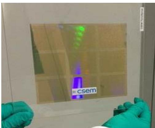
Figure 2: Nanostructures UV replicated by step and repeat process
