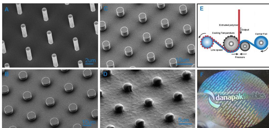
**Figure 1** A-C: The Si masters for replication. D: Structures replicated in polypropylene. E: The schematics of the extrusion coating process and the important parameters. F: Diffractional gratings of  $\frac{1}{2} \mu\text{m}$  that reflect light in a holographic manner, replicated in polypropylene.
