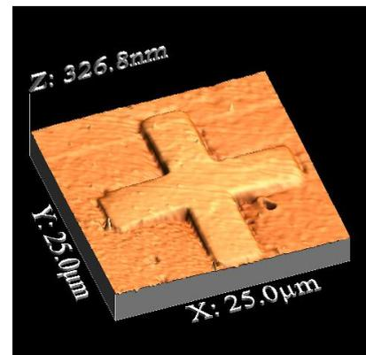
Figure 2: AFM measuring of a nano-mark
