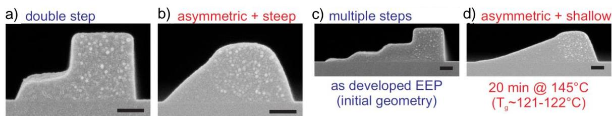
**Figure 2:** a),c): Grayscale topographies after exposure and development. b),d): the same topographies after reflow and re-shaping due to energy self-optimization. (all scale bars 200 nm)
