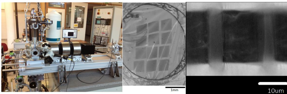
**Figure 1:** Left: PBW system. Middle: Membrane with two  $60 \mu\text{m}$  tape rings for delamination. Right: Cross-sectional micrograph of the membrane.
