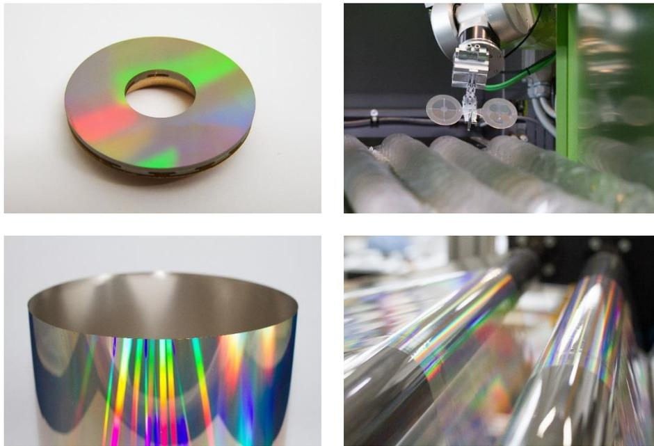
**Figure 1:** Industrial replication of micro and nanostructured films and components, (a) mold insert, (b) injection molding, (c) seamless sleeve, (d) roll-to-roll imprinting
