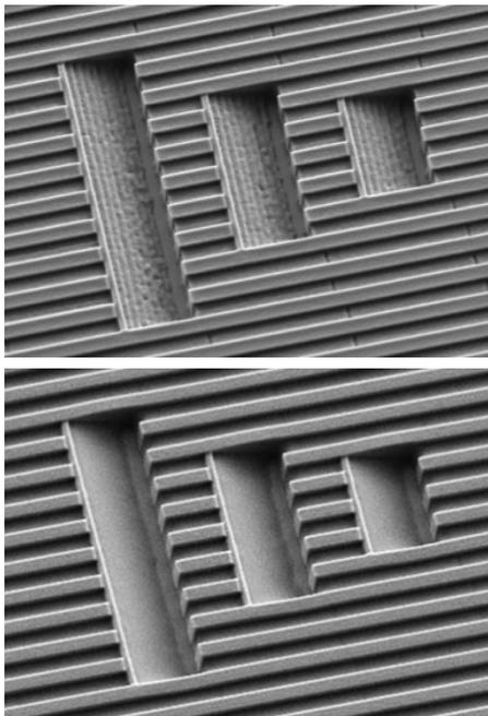
Fig 4: Array of inverted microprisms in pmma before (top) and after (bottom) reflow.
