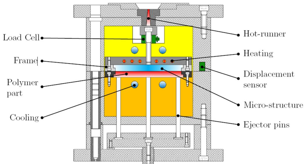
**Figure 1:** Schematic overview of the instrumented injection mold for the measurement of demolding energy [2].
