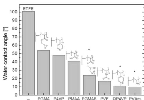
Fig. 3: Adaptation of surface properties of polymers by grafting of polyelectrolytes
