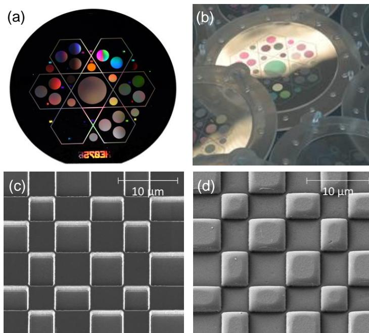
**Figure 1:** (a) 4" Glassy Carbon wafer as a master for plastic injection molding, (b) Cycloolefin copolymer (COC) replica prepared by standard injection molding. (c) SEM image of the GC mold and (d) the corresponding COC replica surface, where the scale bar indicates 10  $\mu\text{m}$ .
