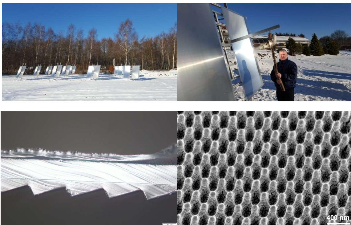
**Figure 1:** Top: First demonstration plant using micro and nanostructured polymer foil to concentrate sunlight. Bottom: Micrographs of the foil structures, Fresnel lens microstructures (left), Highly transparent index gradient nanostructures (right, masters made by Temicon GmbH).
