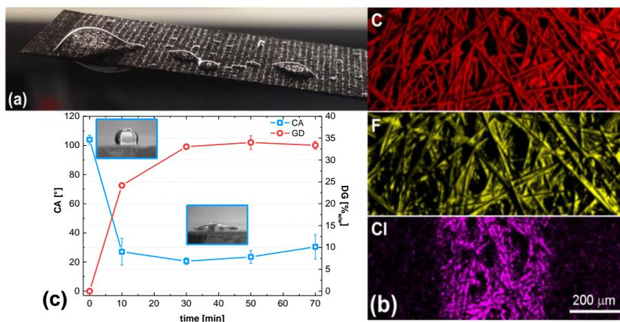
**Figure 1:** (a) Picture of modified carbon paper with pattern wettability. (b) EDX elemental mapping of modified carbon paper (c) Kinetic curve for grafted polymer films showing contact angle (CA) and degree of grafting (DG) versus time.
