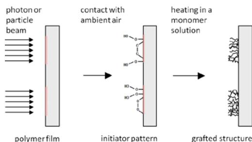
Fig. 1: Scheme of lithographic radiation grafting
