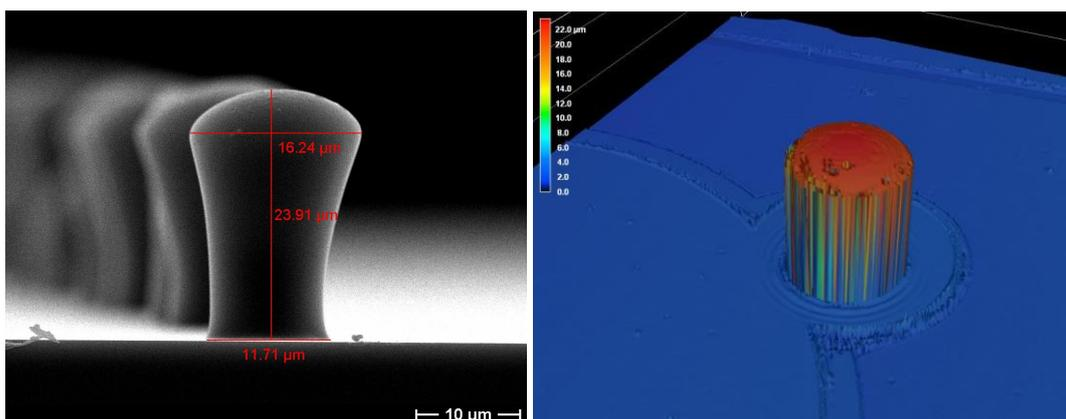
Figure 1: Replication on wafer scale of free-standing micro-lenses
