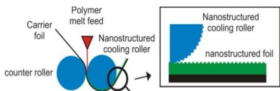
Figure 1: Schematic of R2R-EC. Polymer is heated to a high temperature, such that it achieves a desired low viscosity. Simultaneously, pressure is applied by the counter roller against the structured cooling roller, which is kept well below the solidification temperature of the polymer, forcing the polymer melt deeply into the nanostructures. The structured foil is subsequently wound up.
