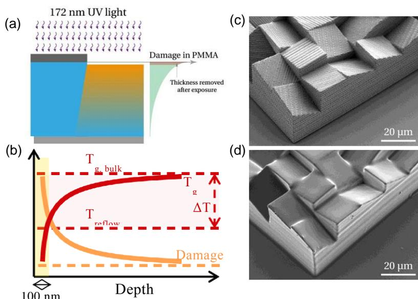
**Figure 1:** (a) Schematic of 172 nm UV exposure to PMMA film. (b) Expected depth profile of the damage in PMMA (orange) and corresponding glass transition temperature dependence (red) for a specific exposure dose. (c) As written micropism array with 2PP. (d) After transfer into PMMA with surface sensitive exposure and reflow for 15 mins at 115°C.
