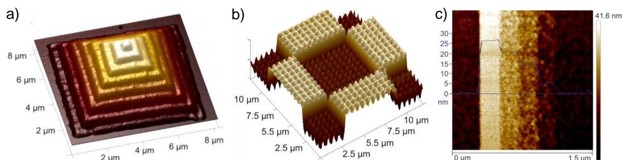
**Figure 1:** Atom force microscopies of grayscale patterns: a) 9-level pattern for diffractive optics, b) hierarchical structure for bio-mimetics, c) 6-level patterns with 6 nm steps.
