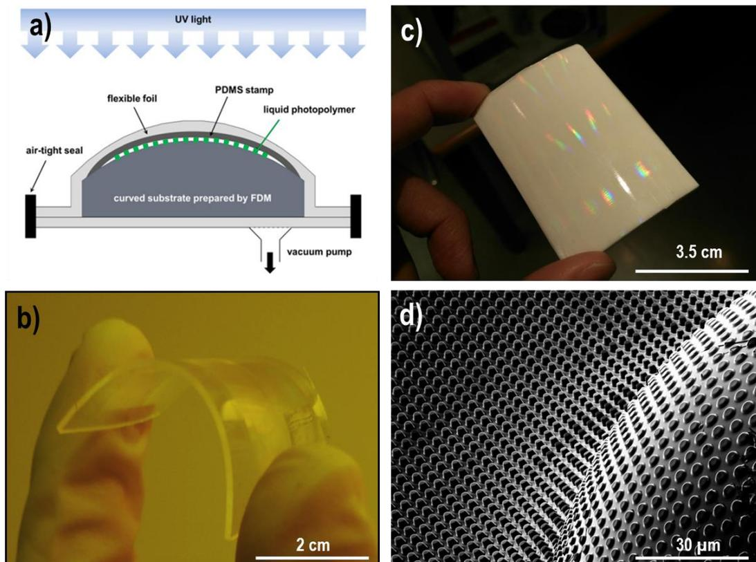
**Figure 1:** a) Schematic drawing showing our setup to perform imprints on curved surfaces. b) Flexible PDMS stamp. c) 3D-printed part curved in one direction with surface structured by nanoimprint lithography. d) Detail of an imprint over a half sphere with 160μm diameter demonstrating the deformation capability of a soft NIL stamp.
