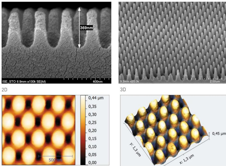
**Figure 2:** Nanostructure (moth-eye structure) with high fidelity after injection molding
