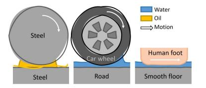
"Systems in which the **elastic deformation** due to the pressure in the lubricating film is not negligible"
