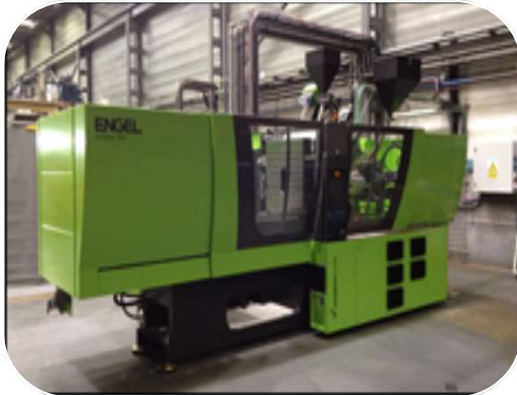
Engel 160 Tn 3K Machine 50 mm / 22 mm / 25 mm Mobile 6 Axis Robot
