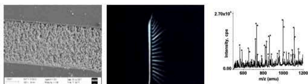
Figure 2: (left to right) SEM of polymer monolith embedded in device for fractionation, sample concentration, enzyme digestion; image of sample fractionation; mass spectrum of Bovine serum albumin digest from microfluidic chip.
